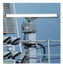
The time taken for a pulse to travel to the object and back can be measured. In this way the distance to the object from the transmitter can be calculated, and its direction can be defined from the detection off the aerial direction. This technique has been extended to the use of computers, which accept data, apply logical processes to the data and supply the results of these processes as the information being sought.
