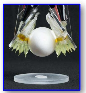
self-healing electrostatic) actuator is strong and versatile but cheap to produce, according to the authors, who only used **a facile heatsealing method** with **inexpensive** commercially available materials to produce this promising technology. **Remarkably**, this actuator is able to lift more than 200 times its weight.
