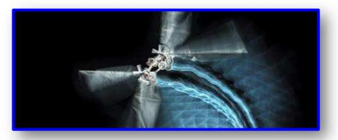
Many **bioinspired robots** serve **a dual purpose**, namely, developing advanced technologies with practical applications and **unveiling** the principles used by nature to build and program living beings. Here, we see the design of a **remarkable**, **tailless**, **untethered**, autonomous, programmable, small (28 g), **flapping**
